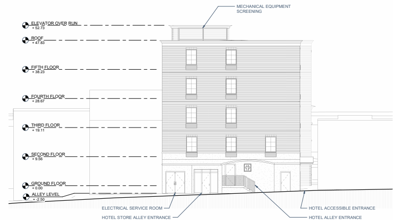
WEST ELEVATION ALLEY
