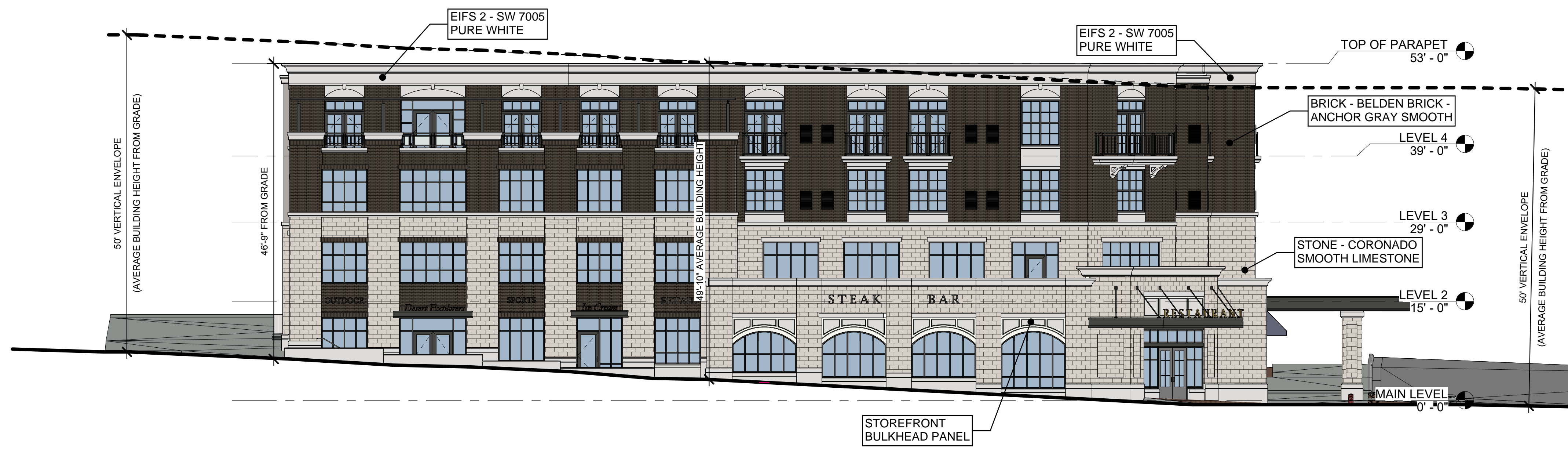
1 NORTH EXTERIOR ELEVATION (GOODWIN STR) SCALE: 3/32" = 1'-0"
