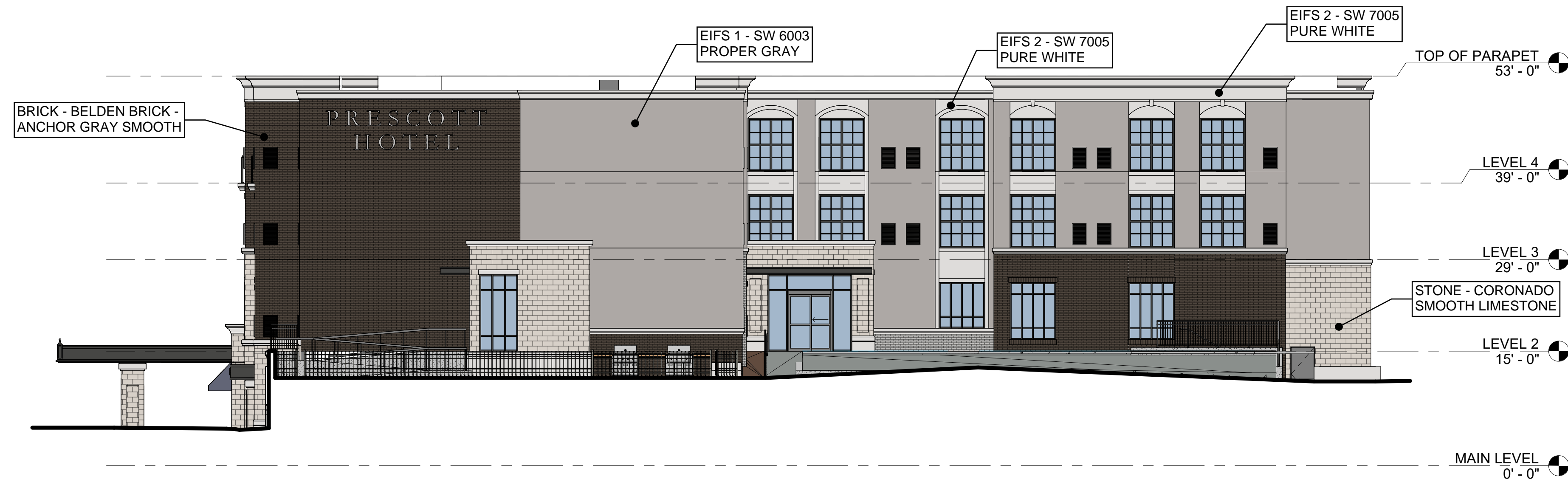
1 SOUTH EXTERIOR ELEVATION SCALE: 3/32" = 1'-0"
