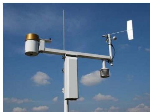
Figure 9. Typical Weather Station for Smart Irrigation
