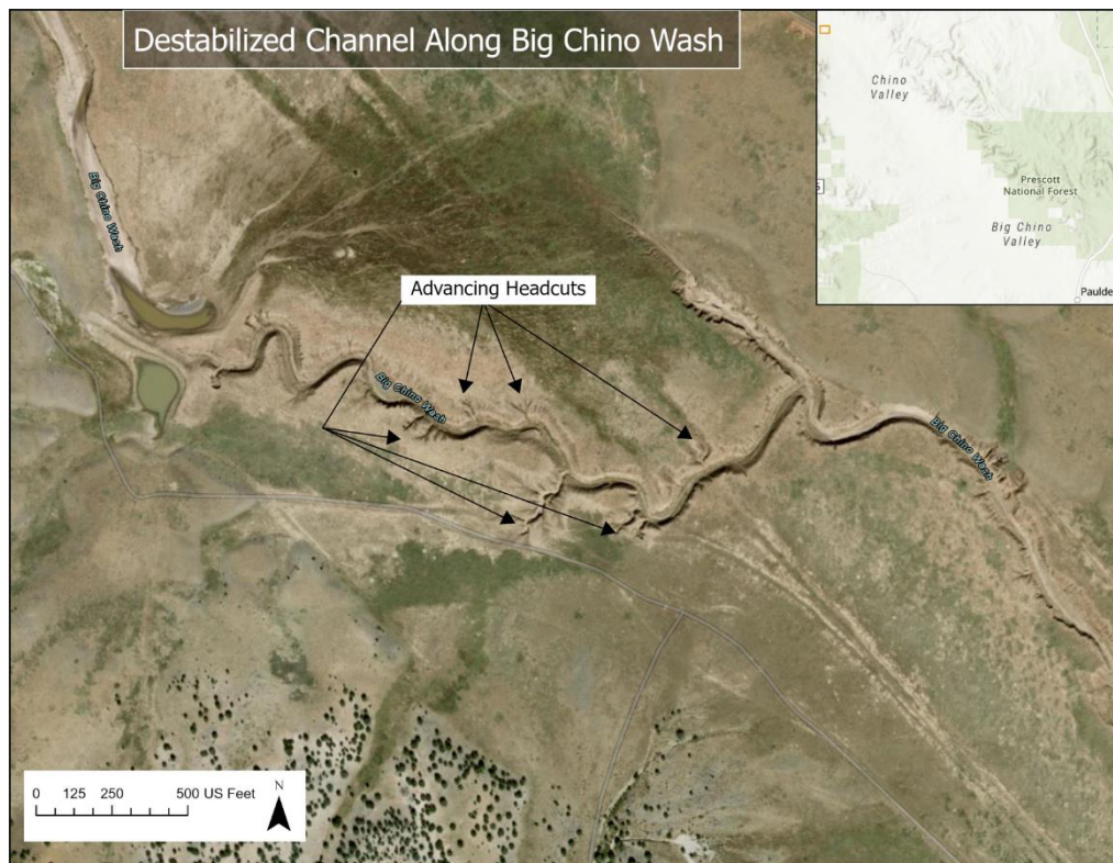
Figure 19 An example of multiple hydrological modifications to Big Chino Wash and advancing headcuts.
