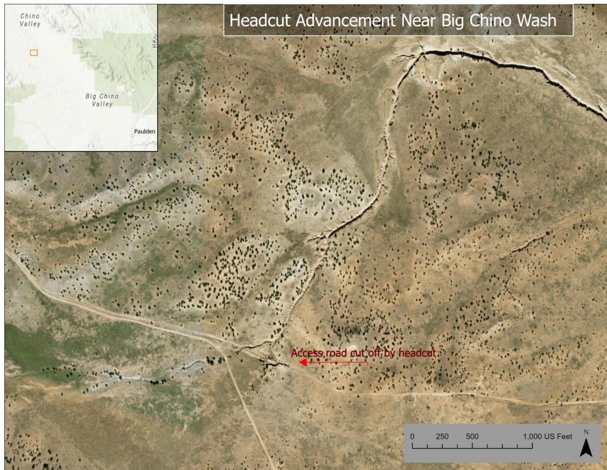
Figure 21 Example of a headcut advancing through K4 Ranch, near Big Chino Wash. The headcut is compromising the access road and moving into productive pasture.
