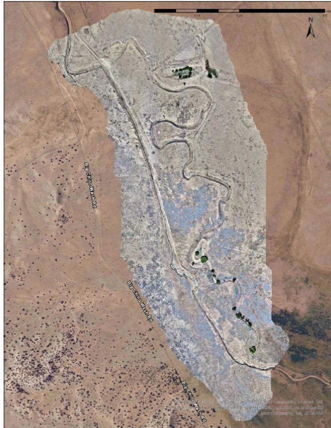
Figure 4. Drone photo of straightened existing channel on the West and the abandoned channel on the east.
